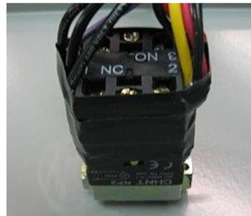
Most Elimia converters use terminal block(s) for all power connections. In the picture below the terminal blocks are labeled and ready for the input power. Don't skimp on wire size! Using wiring that is undersized results in
