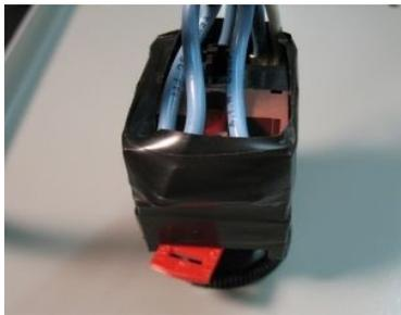
*Some start stop switches are equipped with quick release adapters. These allow you to easily disconnect the pushbuttons from the actuators so that the cover can be removed during installation. Slide the red tabs to release the switches from the panel cover. When you reassembly your cover make sure the red tab is facing down or else your switch functions will be reversed.*
